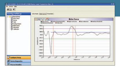
transmitters – typically used where density, vapour and temperature excursions rule out most other alternatives – diagnostics also provide plant engineers with an accurate picture of what the transmitter sees, in terms of obstacles, such as tank baffles etc, by displaying radar echoes in real time.
